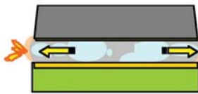
Air bubbles generated by additive reaction capture small voids to force them out.
