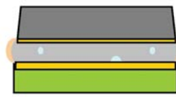
Additive reactions last for a short time and the amount of voids after solidification is less.
