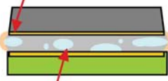
Voids occur due to the reaction with metallic salt MO + RoCOOH \rightarrow (RoCOOH)_2M + H_2O
