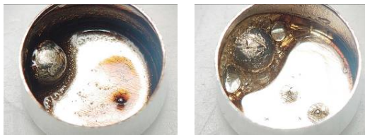
Figure 11: Comparison of flux rosin color after heating at 300°C for lead-free SnAgCu paste showing conventional versus head-in-pillow solder paste performance
