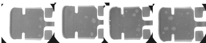
Figure 9: Lead-free Paste C voiding data on the power transistor assembled on different board surface finishes (OSP [2.6% voiding], Pure tin [3.6% voiding], NiAu [5.4% voiding], Sn3Ag0.5Cu HASL[4.6% voiding]).
