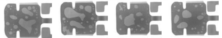
Figure 10: Conventional Lead-free Paste D voiding data on the power transistor assembled on different board surface finishes (OSP [25.2% voiding], Pure tin [35% voiding], NiAu [17.5% voiding], Sn3Ag0.5Cu HASL [17.4% voiding]).
